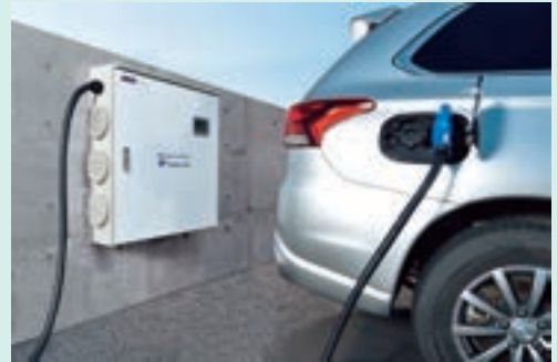
The new model medium-capacity quick charger for electric vehicles
