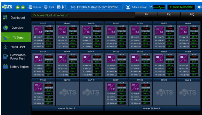
Figure 20. PCSs monitoring display
