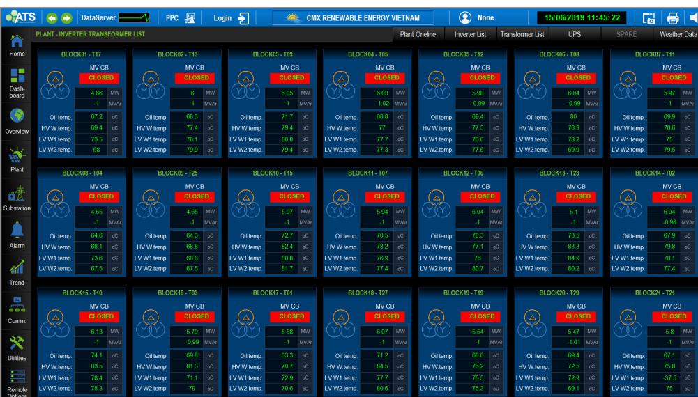
Figure 13. MV transformer monitoring
