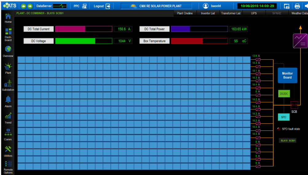
Figure 14. PV String Monitoring
