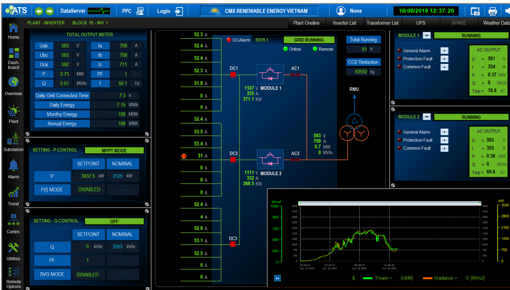
Figure 12. PV Inverter data monitoring and control
