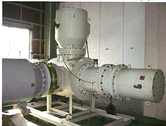
550kV絶縁試験装置 550kV Insulation test equipment
